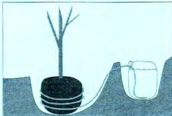
The Wicking Method of Planting and Watering
